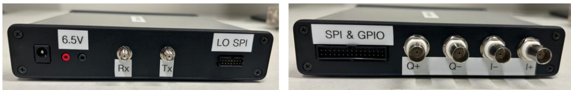
Figure 11 Front and back side of the transceiver box. High frequency input and output (Rx,Tx) and low frequency differential outputs (I+,I-,Q+,Q-) are visible as well as power input (6.5V) and programming interfaces (LO SPI, SPI & GPIO).
