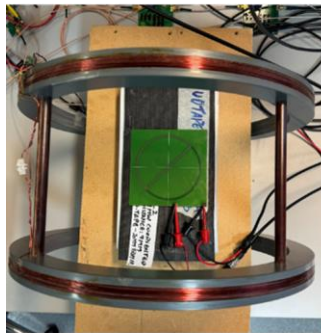
Figure 21 Left: The differential coil system (green square) used for the 1MHz tests. Right: The measurements of the reflection and transmission coefficients show clear peaks originating from the response of the embedded magnetic microwires 3mm below surface in a carbon composite coupon.
