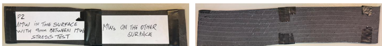
Figure 3 Front and back side of the P2 coupon. Four magnetic microwires with a spacing of 9mm are placed on the back side surface
