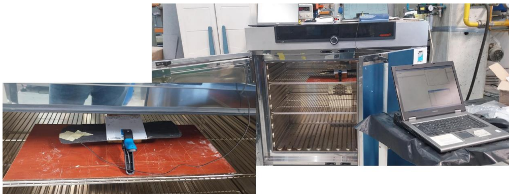
Figure 11: Set-up of the equipment for measuring the effect of temperature on the signal obtained from a carbon specimen with microwires using the PRv3. The specimen is placed in an aging chamber and a thermocouple is placed on the specimen.
