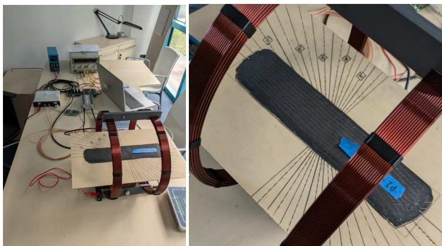
Figure 7: Placement and configuration of the carbon probe in the PRv1 for measurement of the effect of angular variation on the signal.
