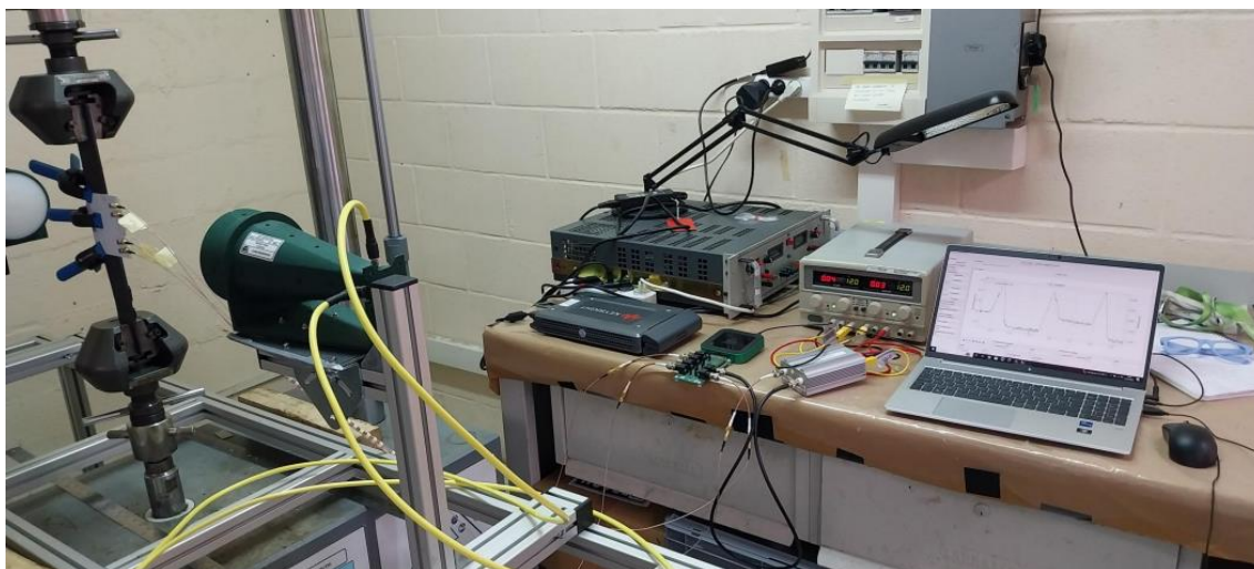
Figure 14: Set-up of the equipment for measuring the effect of tensile force on the signal obtained from the carbon specimen using PRv3
