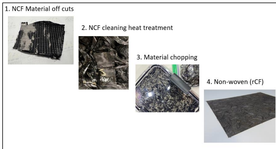
Figure 28. Example of process flow: from collection of the NCF offcuts to conversion into a non-woven.
