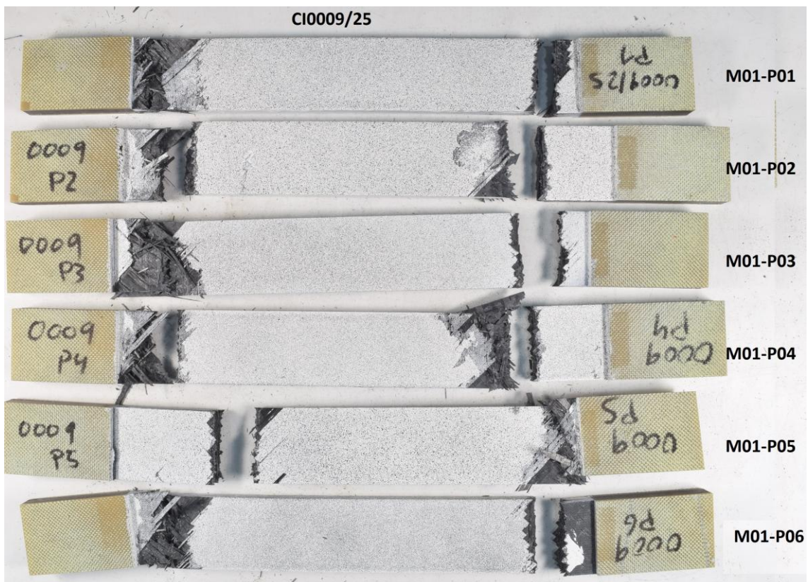
Figure 58. Failure mode for sensorised with microwires coupons – Batch 5. Tensile tests (plain), RT.
