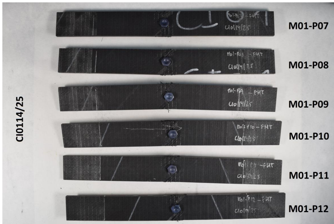
Figure 99. Failure mode for reference coupons – Batch 1. Tensile tests (FHT), LT.
