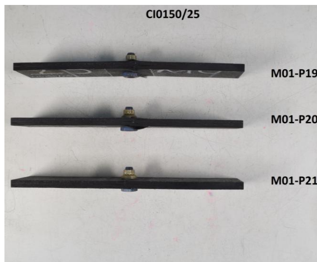
Figure 162. Failure mode for sensorised with microwires coupons – Batch 3. Compression tests (FHC), WET/RT.
