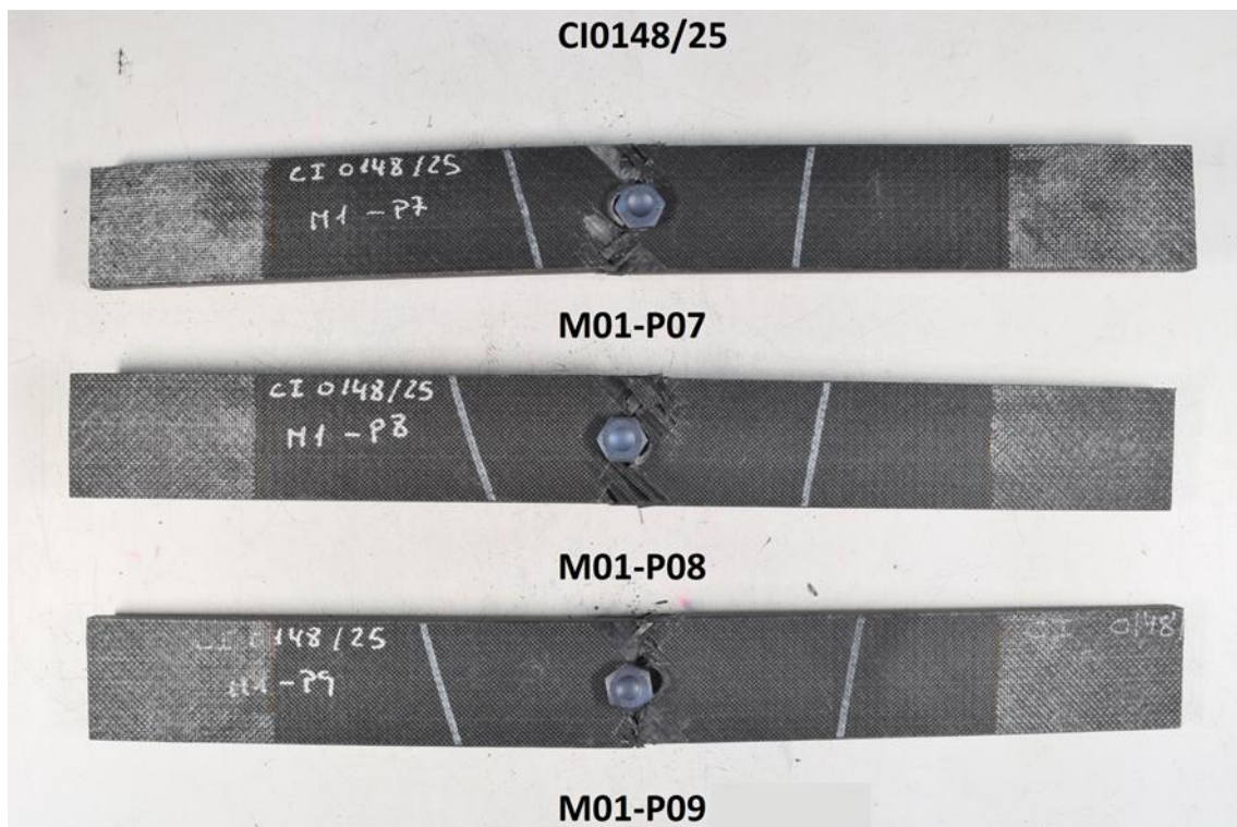
Figure 104. Failure mode for sensorised with microwires coupons – Batch 1. Tensile tests (FHT), WET/RT.
