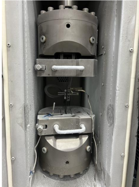
Figure 18. Set-up for low temperature testing
