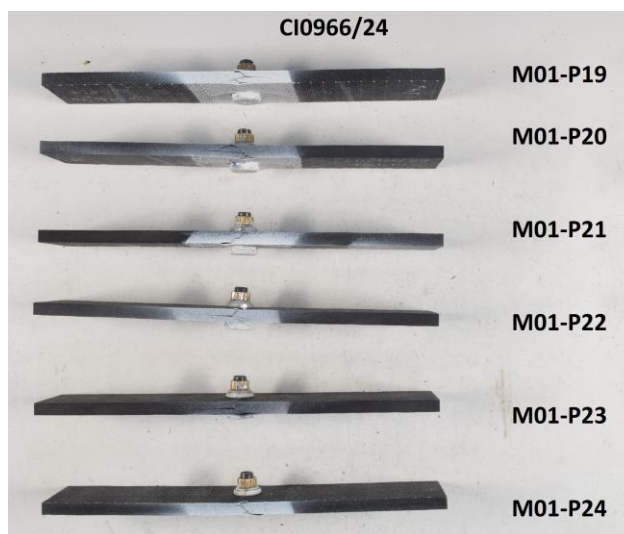
Figure 147. Failure mode for sensorised with microwires coupons – Batch 2. Compression tests (FHC), RT.
