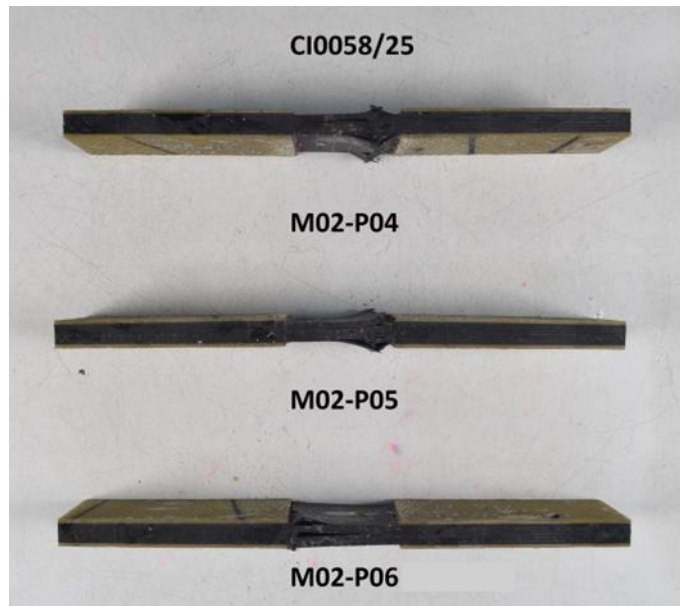
Figure 121. Failure mode for sensorised with microwires coupons – Batch 2. Compression tests (plain), WET/RT.
