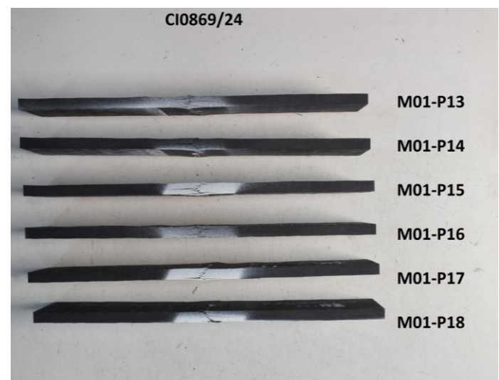
Figure 125. Failure mode for reference coupons – Batch 3. Compression tests (OHC), RT.
