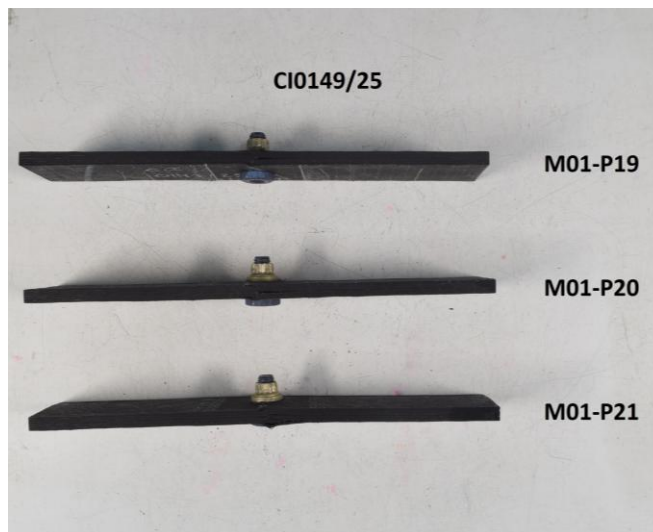
Figure 161. Failure mode for sensorised with microwires coupons – Batch 2. Compression tests (FHC), WET/RT.
