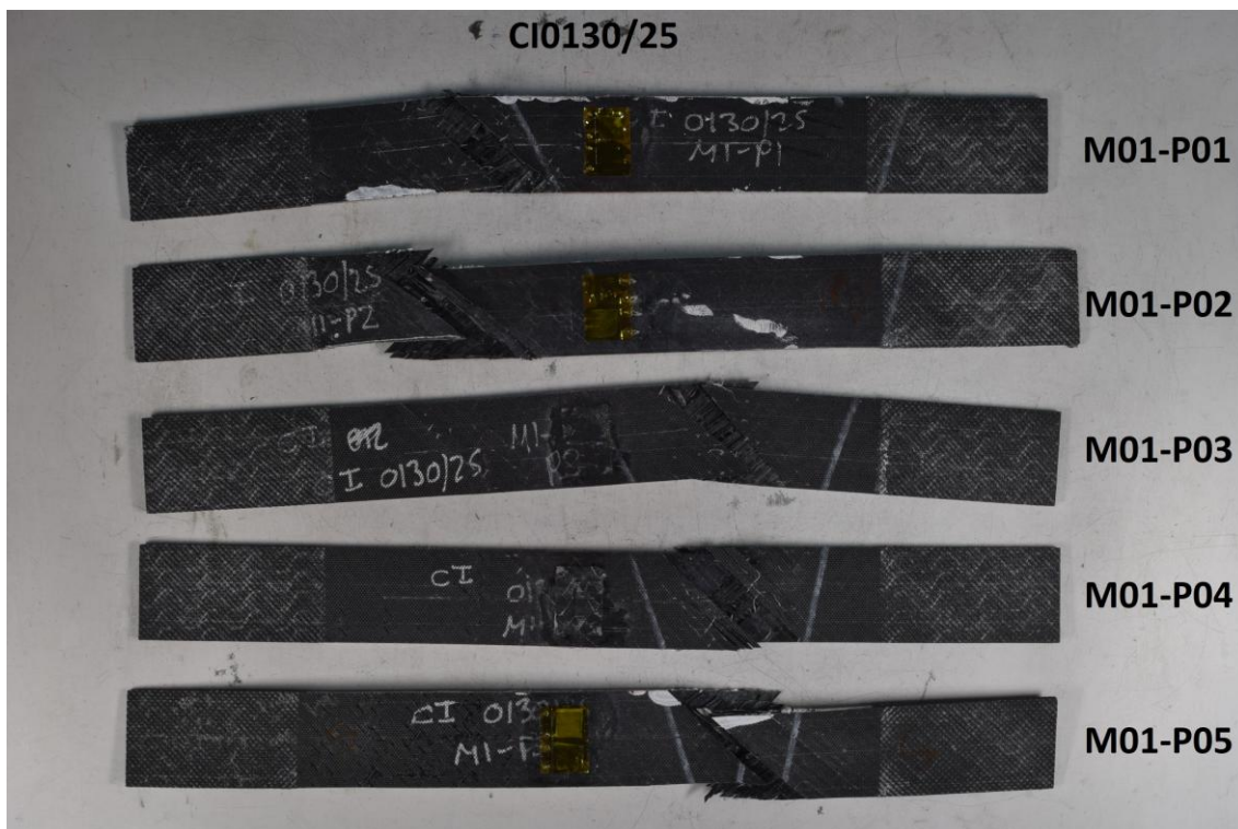
Figure 42. Failure mode for sensorised with microwires coupons – Batch 3. In-plane shear tests, HT.
