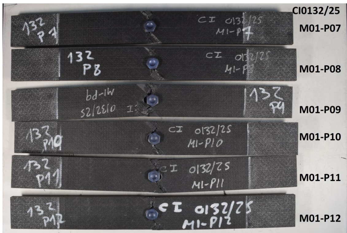
Figure 96. Failure mode for sensorised with microwires coupons – Batch 1. Tensile tests (FHT), HT.
