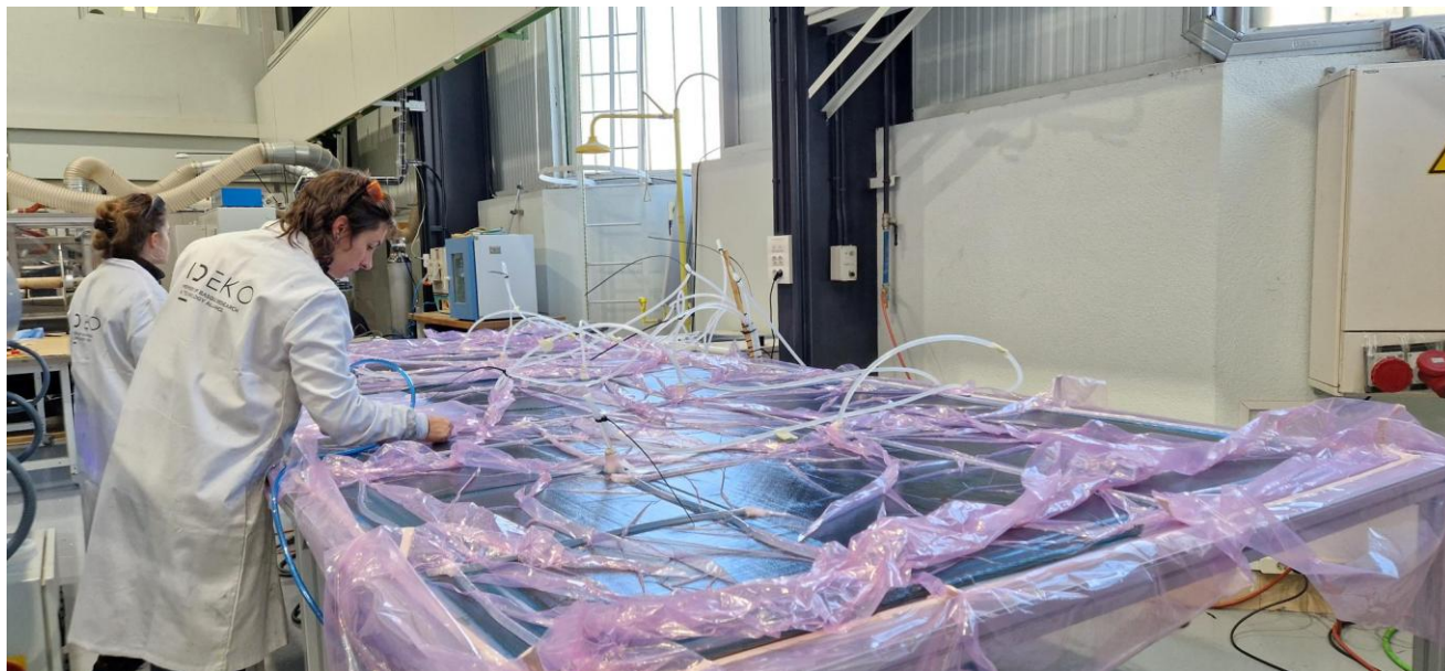
Figure 1. Images from manufacturing process performed at IDEKO. Up: Manual lay up process. Down: Vacuum bags before curing.
