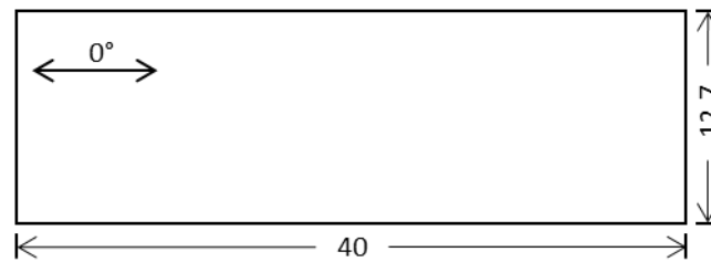
Figure 9. Coupon geometry for flexure test, according to ASTM D790. All dimensions are expressed in mm.
