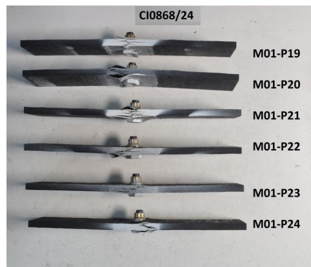
Figure 144. Failure mode for reference coupons – Batch 2. Compression tests (FHC), RT.
