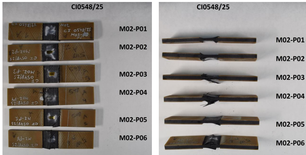
Figure 115. Failure mode for reference coupons – Batch 1. Compression tests (plain), LT.
