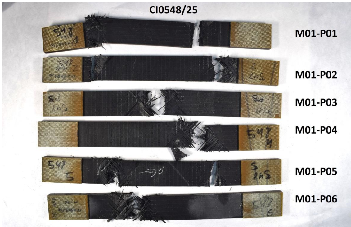
Figure 59. Failure mode for reference coupons – Batch 1. Tensile tests (plain), LT.
