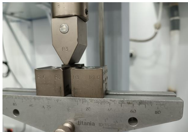
Figure 8. Detail of span in a lap shear strength test.
