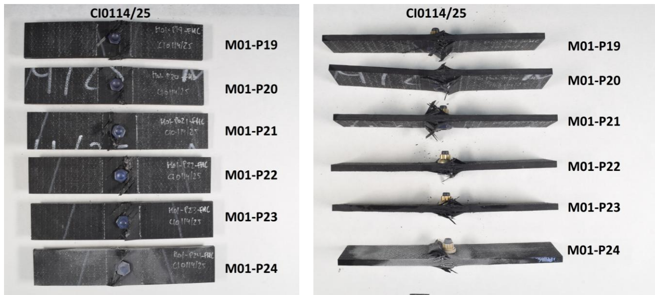
Figure 155. Failure mode for reference coupons – Batch 1. Compression tests (FHC), LT.
