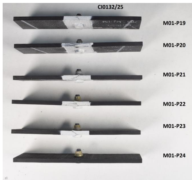
Figure 152. Failure mode for sensorised with microwires coupons – Batch 1. Compression tests (FHC), HT.
