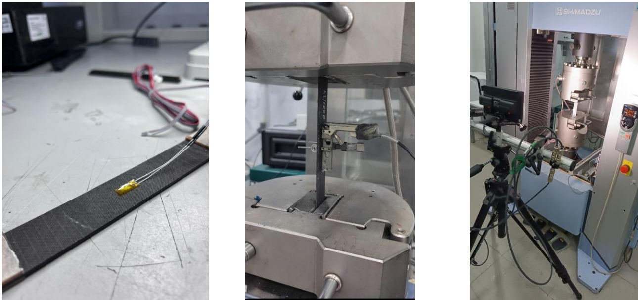
Figure 5. Left: Strain gauge. Centre: Extensometer. Right: DIC
