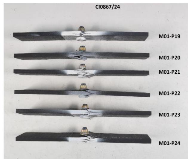
Figure 143. Failure mode for reference coupons – Batch 1. Compression tests (FHC), RT.
