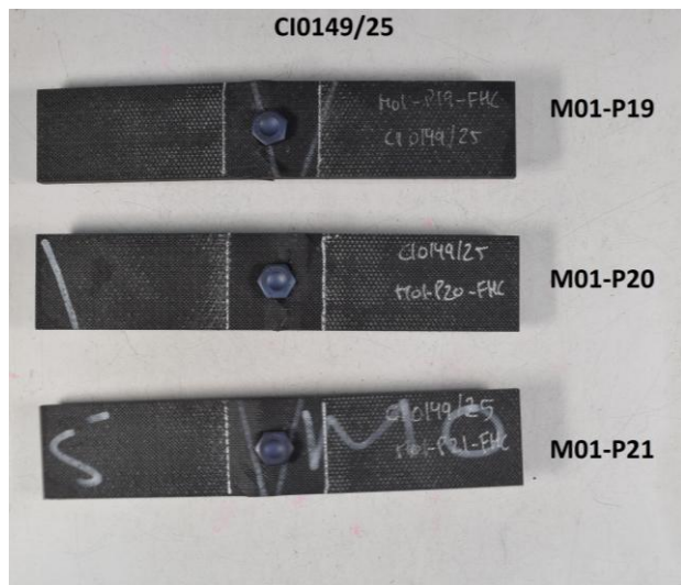
Figure 161. Failure mode for sensorised with microwires coupons – Batch 2. Compression tests (FHC), WET/RT.
