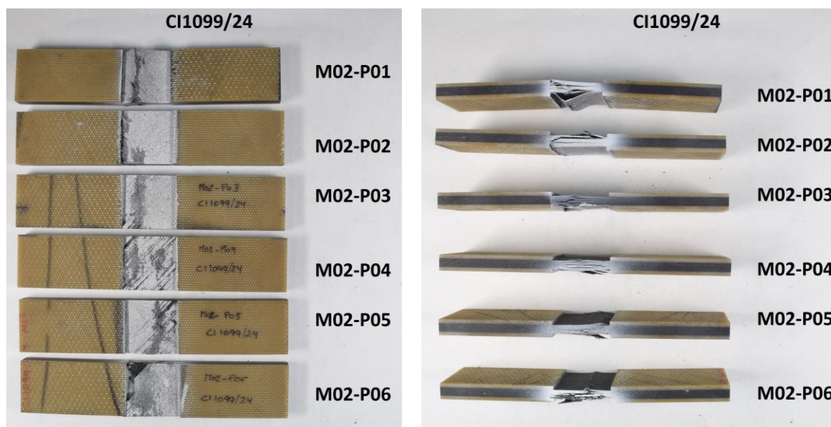
Figure 108. Failure mode for reference coupons – Batch 2. Compression tests (plain), RT.
