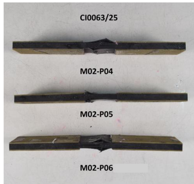
Figure 122. Failure mode for sensorised with microwires coupons – Batch 3. Compression tests (plain), WET/RT.
