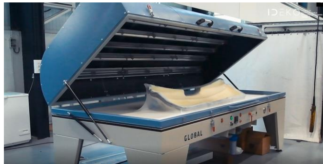
Figure 16. Single membrane heated press used in the preforming process.
