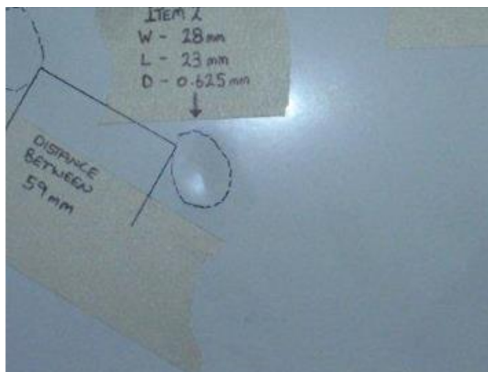
Figure 30. Dent – A surface area which has been depressed with respect to its normal contour. The area boundaries are smooth. Structural integrity is affected by a loss in stiffness of the damaged panel.
