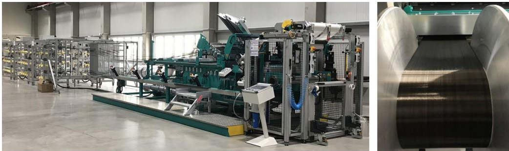
Figure 8. Left: UD Spreading unit. Right: UD Cassette.
