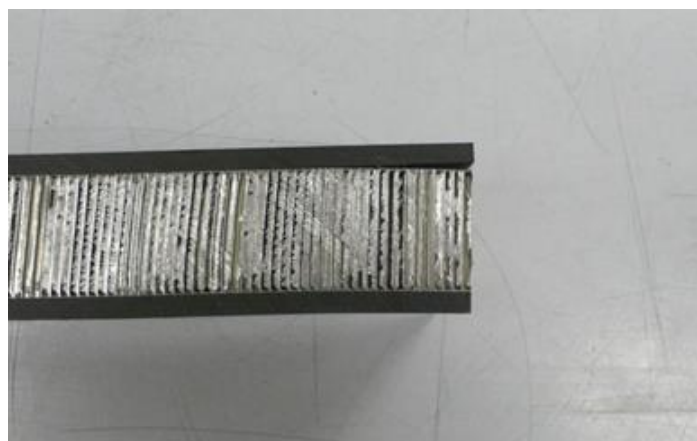
Figure 34. Disbound - A separation of the face sheet from honeycomb core or facing surfaces. Although disbound and delamination are different, they have often been used to describe the same defect.
