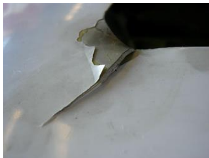
Figure 31. Crack – A fracture or complete separation of the material in one or more of the laminate plies.
